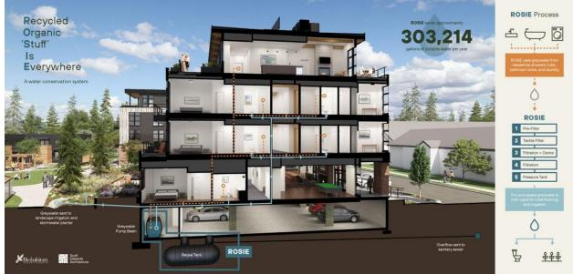
This graphic shows how the ROSIE system works to reclaim greywater from kitchen and laundry usage and recycle it for flush toilets and for irrigation.
